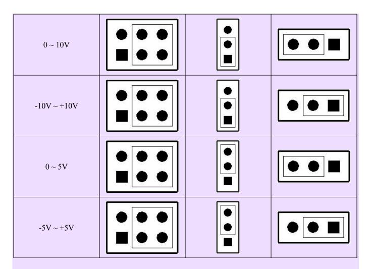
The JP5, JP9, JP6 jumpers are used for CH0 output signal type setting while the JP7, JP10, JP8 jumpers are used for CH1.
