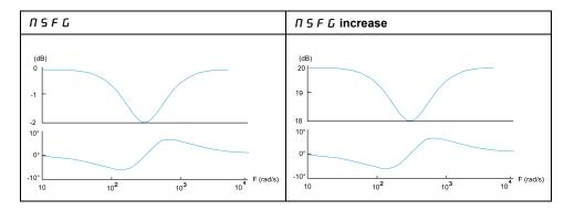
This parameter can be accessed if **[M/S Advanced Filter]**  $\Pi$  5 F E is not set to **[No]**  $\Pi$   $\Pi$ .
