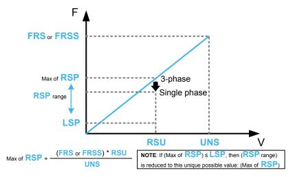
**NOTE:** Compared to a 3–phase power backup supply, the **[Pwr Backup Ref Freq]** r 5 P value may need to be reduced in order to provide the nominal torque with a single phase power backup supply. For more information, you must refer to the application note "Power Backup".
