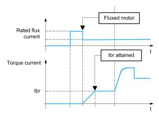
When run command is given, the drive over-fluxes the motor during a short time in order to generate a sufficient motor torque. The level of the torque is set with the
