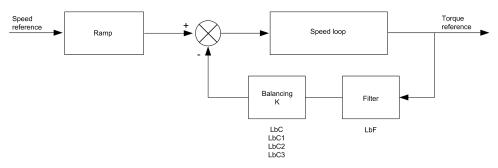
The load sharing factor K is determined by the torque and speed, with two factors K1 and K2 ( $K = K1 \times K2$ ).
