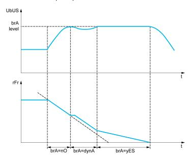
Activating this function automatically adapts the deceleration ramp, if this has been set at a too low value according to the inertia of the load, which can cause an overvoltage detected error.
