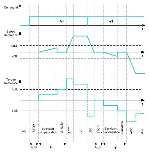
Regulate 0Hz speed at direction change (UC-3)
