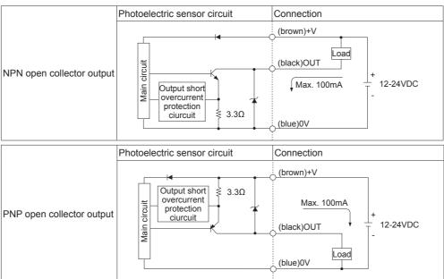
XIf short-circuit the control output terminal or supply current over the rated specification, normal control signal is not output due to the output short over current protection circuit.
