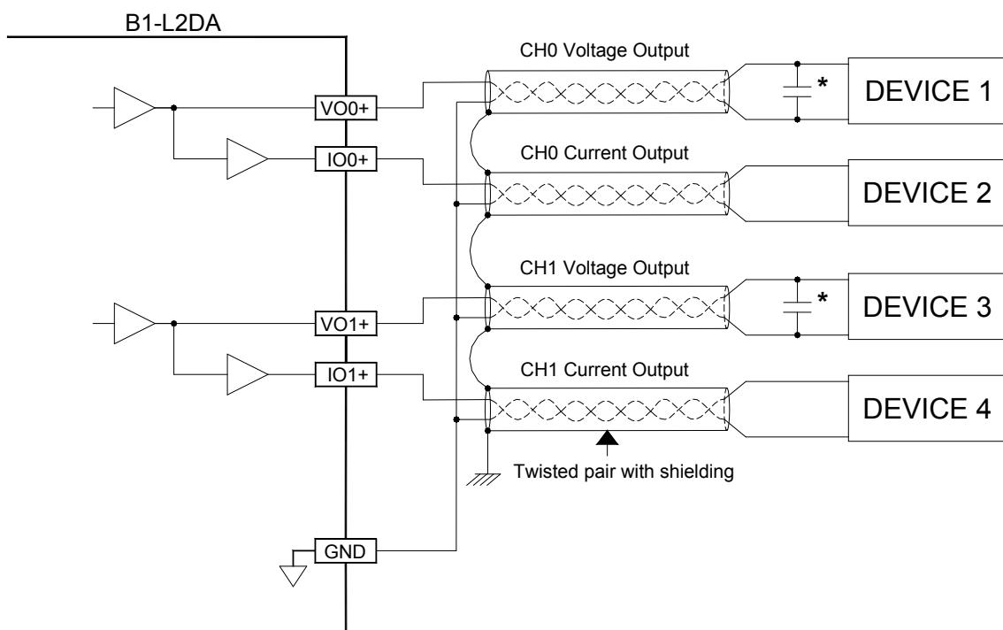
\*0.1~0.47uF capacitor (to filter noise).....Advice to install, but not necessary!!
