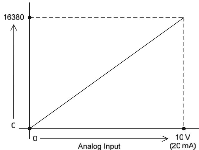
Figure 2 : Analog Output Characteristics Curve
